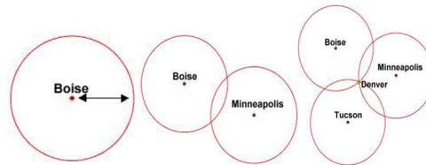
Figure 2. Principle of trilateration in 2-D space
