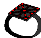
Fig 7. Programmable HIOX ring with 16-segment LED display.
